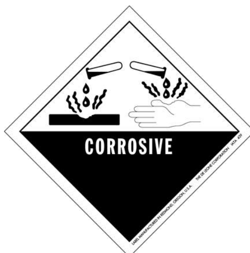
Figure 3. Label model No. 8 [Class 8 – Corrosive substances]
