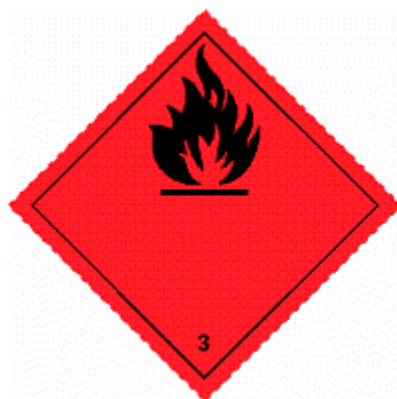
Figure 1. Label model No. 3 [Class 3 – Flammable liquids]
