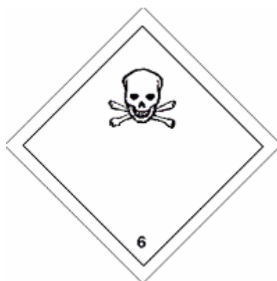
Figure 2. Label model No. 6.1 [Class 6 – Toxic substances]
