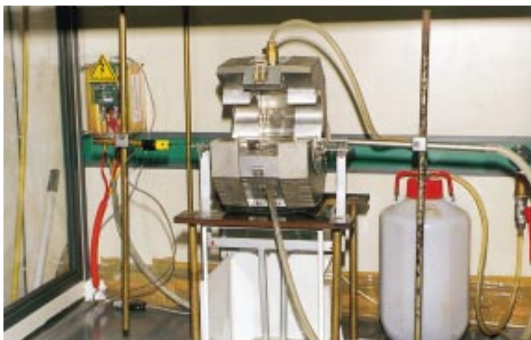
Figure 1: A bench scale system for the determination of the chemical kinetics of biomass reactions.
